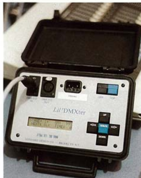
Lil'DMXter: most useful test tool for electricians.
