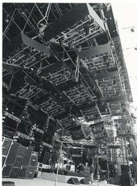
The Vari*Lite pods overhead with 4kW of Clair Bros monitors on stage.
