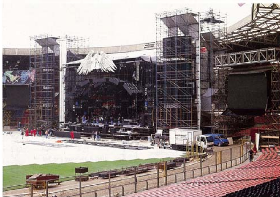
The three technical facets of the show: video monitor, PA stacks and stage lighting rig.
